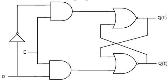
This circuit has single input D and two outputs  $Q_t$  &  $Q_t'$ . D Latch is obtained from SR Latch by placing an inverter between S amp; R inputs and connect D input to S. That means we eliminated the combinations of S & R are of same value.
