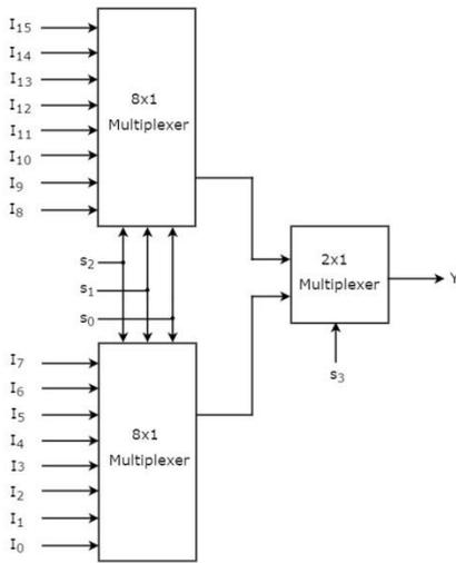
The **same selection lines**,  $s_2$ ,  $s_1$  &  $s_0$  are applied to both 8x1 Multiplexers. The data inputs of upper 8x1 Multiplexer are  $I_{15}$  to  $I_8$  and the data inputs of lower 8x1 Multiplexer are  $I_7$  to  $I_0$ . Therefore, each 8x1 Multiplexer produces an output based on the values of selection lines,  $s_2$ ,  $s_1$  &  $s_0$ .
