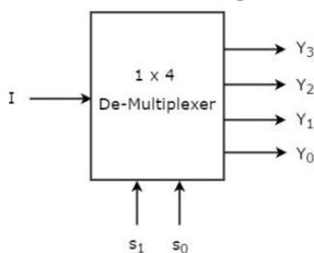
The single input 'I' will be connected to one of the four outputs,  $Y_3$  to  $Y_0$  based on the values of selection lines  $s_1$  &  $s_0$ . The **Truth table** of 1x4 De-Multiplexer is shown below.
