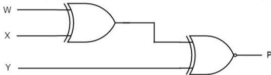
The above circuit diagram consists of Ex-OR gate in first level and Ex-NOR gate in second level. Since the odd parity is just opposite to even parity, we can place an inverter at the output of even parity generator. In that case, the first and second levels contain an ExOR gate in each level and third level consist of an inverter.
