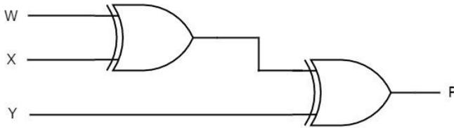
This circuit consists of two **Exclusive-OR gates** having two inputs each. First Exclusive-OR gate having two inputs W & X and produces an output  $W \oplus X$ . This output is given as one input of second Exclusive-OR gate. The other input of this second Exclusive-OR gate is Y and produces an output of  $W \oplus X \oplus Y$ .
