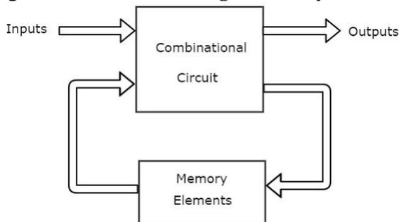
This sequential circuit contains a set of inputs and outputs. The outputs of sequential circuit depends not only on the combination of present inputs but also on the previous outputs. Previous output is nothing but the **present state**. Therefore, sequential circuits contain combinational circuits along with memory storage elements. Some sequential circuits may not contain combinational circuits, but only memory elements.
