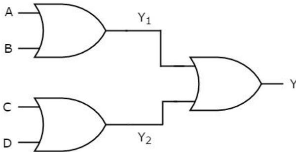
We will get the outputs of first level logic gates as  $Y_1=A+B$  and  $Y_2=C+D$ .
