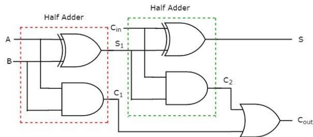
This adder is called as **Full adder** because for implementing one Full adder, we require two Half adders and one OR gate. If  $C_{in}$  is zero, then Full adder becomes Half adder. We can verify it easily from the above circuit diagram or from the Boolean functions of outputs of Full adder.
