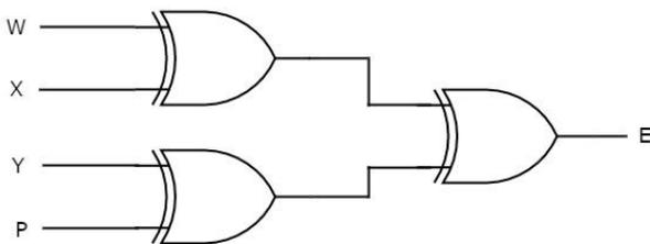
This circuit consists of three **Exclusive-OR gates** having two inputs each. The first level gates produce outputs of  $W\oplus X$  &  $Y\oplus P$ . The Exclusive-OR gate, which is in second level produces an output of  $W\oplus X\oplus Y\oplus P$
