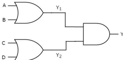
Previously, we got the outputs of first level logic gates as  $Y_1=A+B$  and  $Y_2=C+D$ .
