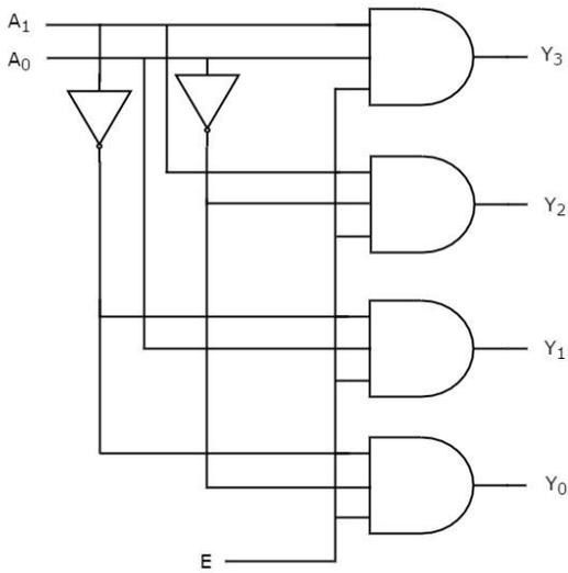
Therefore, the outputs of 2 to 4 decoder are nothing but the **min terms** of two input variables  $A_1$  &  $A_0$ , when enable, E is equal to one. If enable, E is zero, then all the outputs of decoder will be equal to zero.
