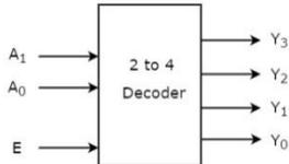
One of these four outputs will be ‘1’ for each combination of inputs when enable, E is ‘1’. The **Truth table** of 2 to 4 decoder is shown below.
