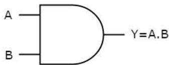
This AND gate produces an output Y, which is the **logical AND** of two inputs A, B. Similarly, if there are ‘n’ inputs, then the AND gate produces an output, which is the logical AND of all those inputs. That means, the output of AND gate will be ‘1’, when all the inputs are ‘1’.
