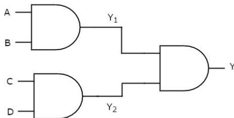
We will get the outputs of first level logic gates as  $Y_1 = AB$  and  $Y_2 = CD$
