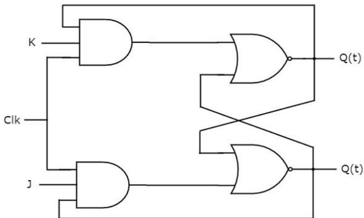
This circuit has two inputs J & K and two outputs  $Q_{tt}$  &  $Q_{tt}'$ . The operation of JK flip-flop is similar to SR flip-flop. Here, we considered the inputs of SR flip-flop as  $S = J Q_t'$  and  $R = K Q_t$  in order to utilize the modified SR flip-flop for 4 combinations of inputs.
