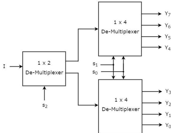
The common **selection lines**,  $s_1$  &  $s_0$  are applied to both 1x4 De-Multiplexers. The outputs of upper 1x4 De-Multiplexer are  $Y_7$  to  $Y_4$  and the outputs of lower 1x4 De-Multiplexer are  $Y_3$  to  $Y_0$ .
