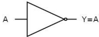
This NOT gate produces an output  $Y$ , which is the **complement** of input, A.
