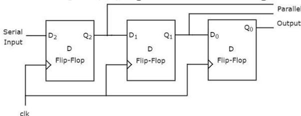
This circuit consists of three D flip-flops, which are cascaded. That means, output of one D flip-flop is connected as the input of next D flip-flop. All these flip-flops are synchronous with each other since, the same clock signal is applied to each one.
