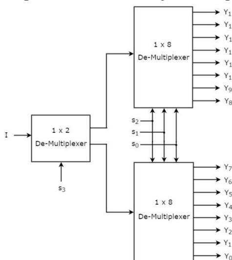
The common **selection lines**  $s_2$ ,  $s_1$  &  $s_0$  are applied to both 1x8 De-Multiplexers. The outputs of upper 1x8 De-Multiplexer are  $Y_{15}$  to  $Y_8$  and the outputs of lower 1x8 De-Multiplexer are  $Y_7$  to  $Y_0$ .
