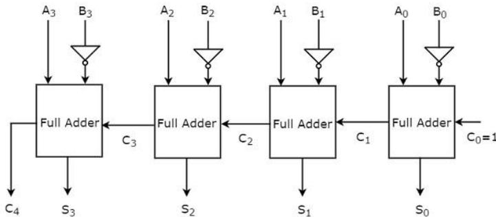
This 4-bit binary subtractor produces an output, which is having at most 5 bits. If Binary number A is greater than Binary number B, then MSB of the output is zero and the remaining bits hold the magnitude of A-B. If Binary number A is less than Binary number B, then MSB of the output is one. So, take the 2's complement of output in order to get the magnitude of A-B.
