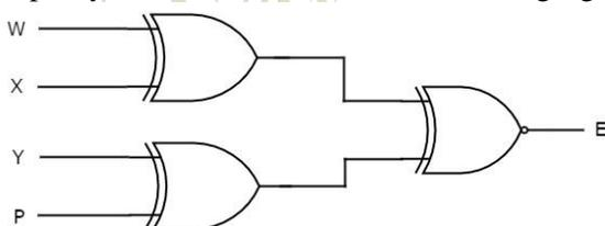
The above circuit diagram consists of Ex-OR gates in first level and Ex-NOR gate in second level. Since the odd parity is just opposite to even parity, we can place an inverter at the output of even parity checker. In that case, the first, second and third levels contain two Ex-OR gates, one Ex-OR gate and one inverter respectively.
