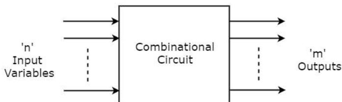
This combinational circuit has 'n' input variables and 'm' outputs. Each combination of input variables will affect the outputs.
