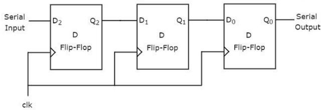
This block diagram consists of three D flip-flops, which are **cascaded**. That means, output of one D flip-flop is connected as the input of next D flip-flop. All these flip-flops are synchronous with each other since, the same clock signal is applied to each one.
