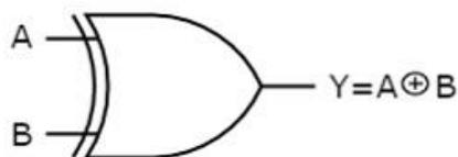
Ex-OR gate operation is similar to that of OR gate, except for few combinations of inputs. That's why the Ex-OR gate symbol is represented like that. The output of Ex-OR gate is '1', when odd number of ones present at the inputs. Hence, the output of Ex-OR gate is also called as an **odd function**.
