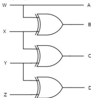
Since the outputs depend only on the present inputs, this 4-bit Binary code to Gray code converter is a combinational circuit. Similarly, you can implement other code converters.
