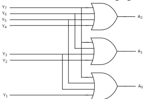
The above circuit diagram contains three 4-input OR gates. These OR gates encode the eight inputs with three bits.
