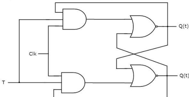
This circuit has single input T and two outputs  $Q_t$  &  $Q_t'$ . The operation of T flip-flop is same as that of JK flip-flop. Here, we considered the inputs of JK flip-flop as  $J = T$  and  $K = T$  in order to utilize the modified JK flip-flop for 2 combinations of inputs. So, we eliminated the other two combinations of J & K, for which those two values are complement to each other in T flip-flop.
