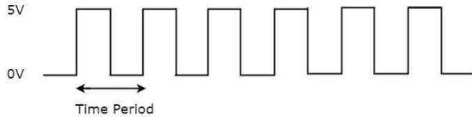
In the above figure, square wave is considered as clock signal. This signal stays at logic High 5V for some time and stays at logic Low 0V for equal amount of time. This pattern repeats with some time period. In this case, the **time period** will be equal to either twice of ON time or twice of OFF time.
