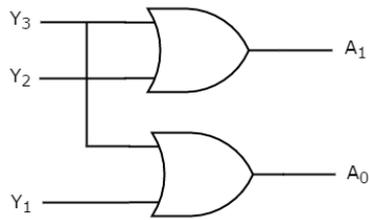
The above circuit diagram contains two OR gates. These OR gates encode the four inputs with two bits
