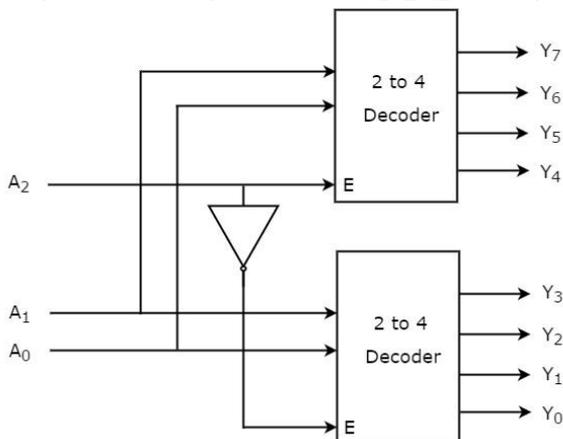
The parallel inputs  $A_1$  &  $A_0$  are applied to each 2 to 4 decoder. The complement of input  $A_2$  is connected to Enable, E of lower 2 to 4 decoder in order to get the outputs,  $Y_3$  to  $Y_0$ . These are the **lower four min terms**. The input,  $A_2$  is directly connected to Enable, E of upper 2 to 4 decoder in order to get the outputs,  $Y_7$  to  $Y_4$ . These are the **higher four min terms**.
