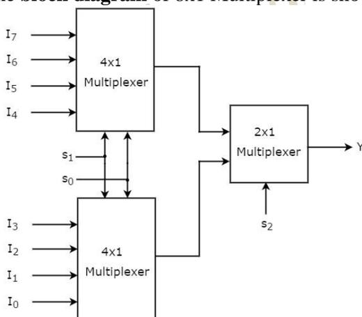
The same **selection lines**,  $s_1$  &  $s_0$  are applied to both 4x1 Multiplexers. The data inputs of upper 4x1 Multiplexer are  $I_7$  to  $I_4$  and the data inputs of lower 4x1 Multiplexer are  $I_3$  to  $I_0$ . Therefore, each 4x1 Multiplexer produces an output based on the values of selection lines,  $s_1$  &  $s_0$ .
