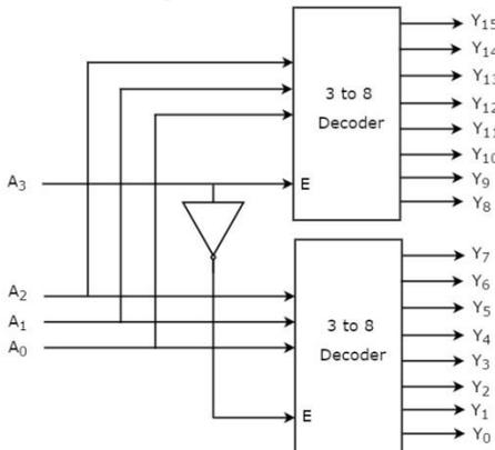
The parallel inputs  $A_2, A_1$  &  $A_0$  are applied to each 3 to 8 decoder. The complement of input,  $A_3$  is connected to Enable,  $E$  of lower 3 to 8 decoder in order to get the outputs,  $Y_7$  to  $Y_0$ . These are the **lower eight min terms**. The input,  $A_3$  is directly connected to Enable,  $E$  of upper 3 to 8 decoder in order to get the outputs,  $Y_{15}$  to  $Y_8$ . These are the **higher eight min terms**.
