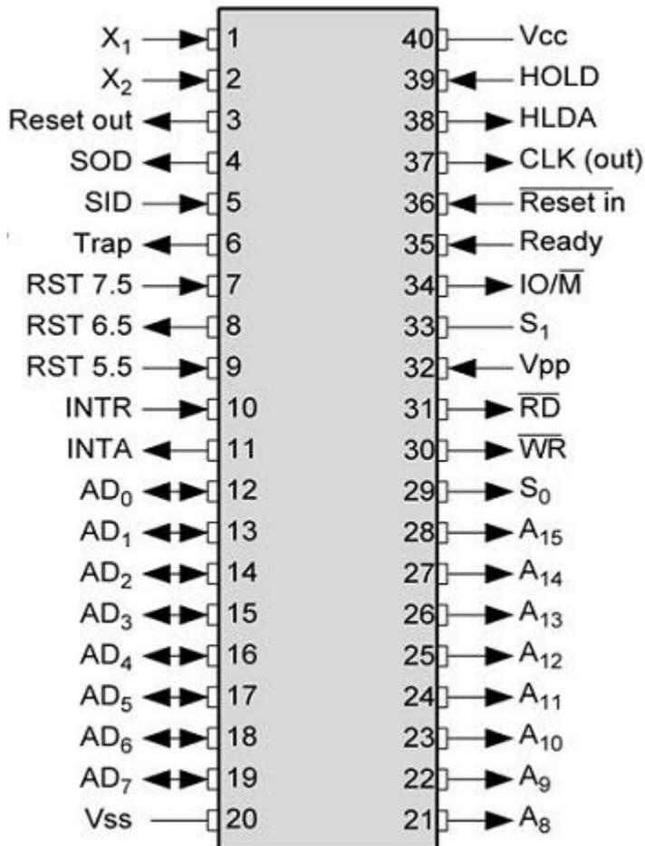
The pins of a 8085 microprocessor can be classified into seven groups –
