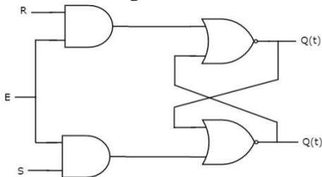
This circuit has two inputs S & R and two outputs  $Q_t$  &  $Q_t'$ . The **upper NOR gate** has two inputs R & complement of present state,  $Q_t'$  and produces next state,  $Q_{t+1}$  when enable, E is '1'.
