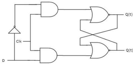
This circuit has single input D and two outputs  $Q_t$  &  $Q_t'$ . The operation of D flip-flop is similar to D Latch. But, this flip-flop affects the outputs only when positive transition of the clock signal is applied instead of active enable. The following table shows the **state table** of D flip-flop.
