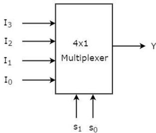
One of these 4 inputs will be connected to the output based on the combination of inputs present at these two selection lines. **Truth table** of 4x1 Multiplexer is shown below.
