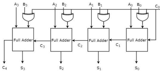
If initial carry,  $C_0$  is zero, then each full adder gets the normal bits of binary numbers A & B. So, the 4-bit binary adder / subtractor produces an output, which is the **addition of two binary numbers A & B**.
