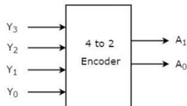
At any time, only one of these 4 inputs can be '1' in order to get the respective binary code at the output. The **Truth table** of 4 to 2 encoder is shown below.
