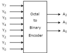
At any time, only one of these eight inputs can be '1' in order to get the respective binary code. The **Truth table** of octal to binary encoder is shown below.
