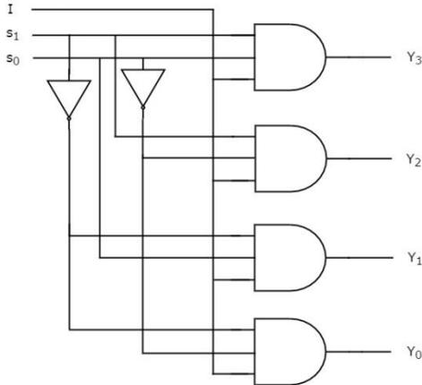
We can easily understand the operation of the above circuit. Similarly, you can implement 1x8 De-Multiplexer and 1x16 De-Multiplexer by following the same procedure.
