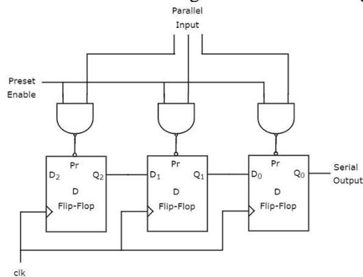
This circuit consists of three D flip-flops, which are cascaded. That means, output of one D flip-flop is connected as the input of next D flip-flop. All these flip-flops are synchronous with each other since, the same clock signal is applied to each one.
