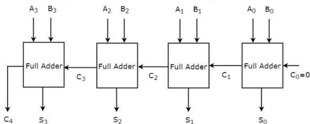
Here, the 4 Full adders are cascaded. Each Full adder is getting the respective bits of two parallel inputs  $A$  &  $B$ . The carry output of one Full adder will be the carry input of subsequent higher order Full adder. This 4-bit binary adder produces the resultant sum having at most 5 bits. So, carry out of last stage Full adder will be the MSB.
